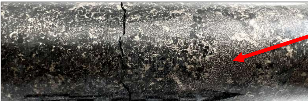
Figure 9: Core from the Camp Zone deposit area drill hole CZ2025-01 – Near surface net-textured to semi-massive mineralization from around 32m to 81m depth.
