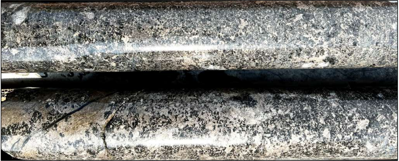
Figure 8: Core from the Camp Zone deposit area drill hole CZ2025-01 – Near surface net-textured to semi-massive mineralization from around 32m to 81m depth.
