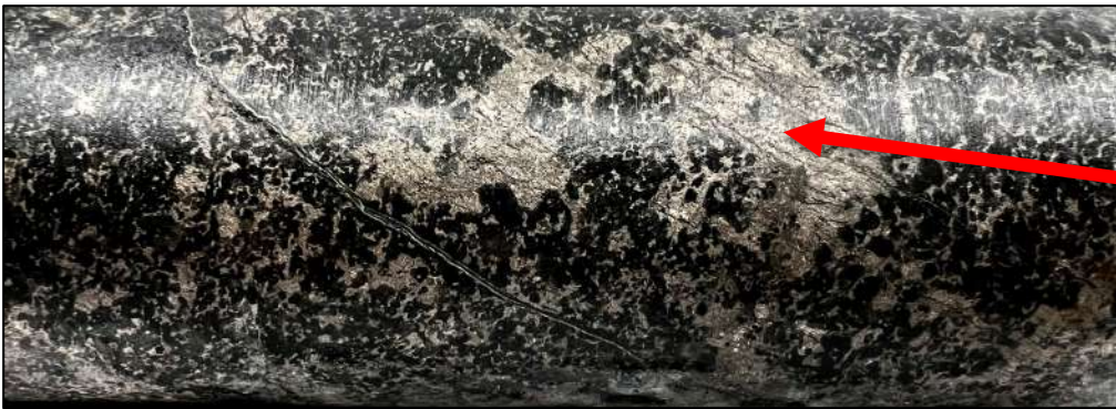
Figure 8: Core from the Camp Zone deposit area drill hole CZ2025-01 – Near surface net-textured to semi-massive mineralization from around 32m to 81m depth.
