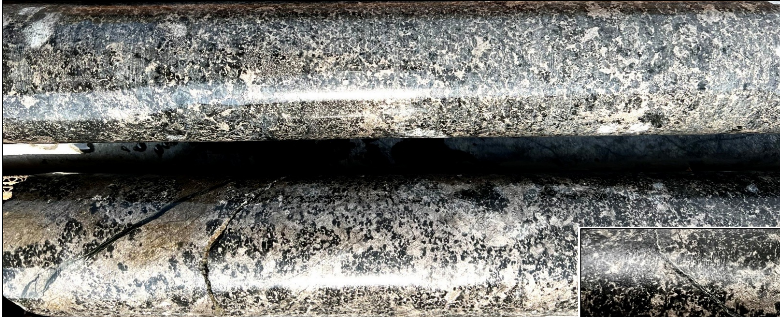
Core from Camp Zone drill hole CZ2025-01: Near surface (at 32m to 81m depth) net-textured to semi-massive mineralization.
